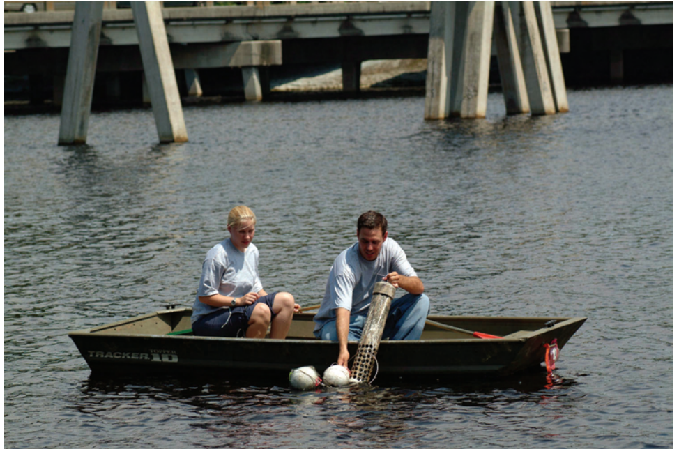
Deploying a 'gator-proofed' sonde near Tampa.
