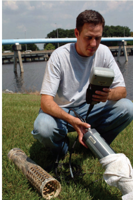
A BRA analyst calibrates a YSI sonde in the field.
